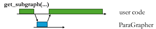
Figure 2: A synchronous (blocking) call. The library parallelizes loading/decompression while user is waiting for receiving the requested graph/subgraph all at once .
